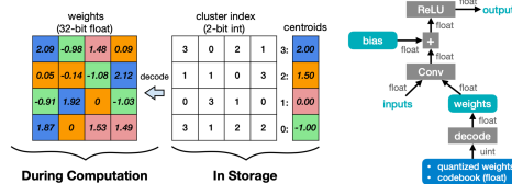
Figure 10: Inference: indices and codebook are stored, decoded to FP32, then used in a standard matmul.
