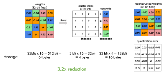
Figure 6: Used by Xuanbin and Yinuo; Clustering example, clustering with K = 4 centroids: indices, codebook, reconstruction, and per-element error.
